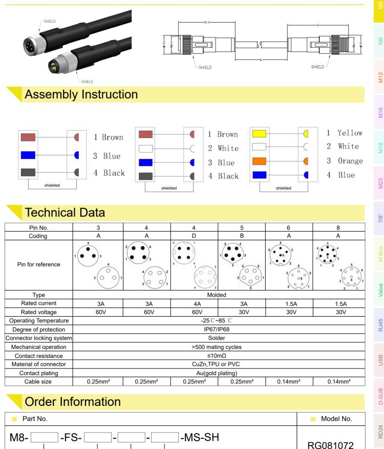
Remark:Shielded wire contact the metal shell .Contact us any time if you have custom requirements.
